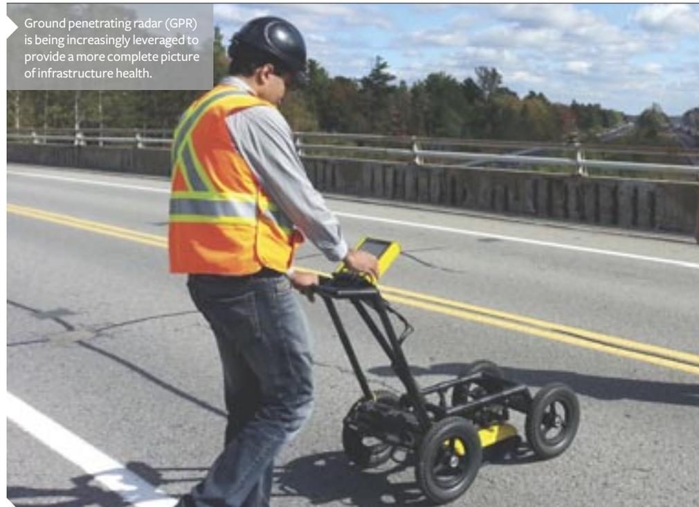
Ground penetrating radar (GPR) is being increasingly leveraged to provide a more complete picture of infrastructure health.
