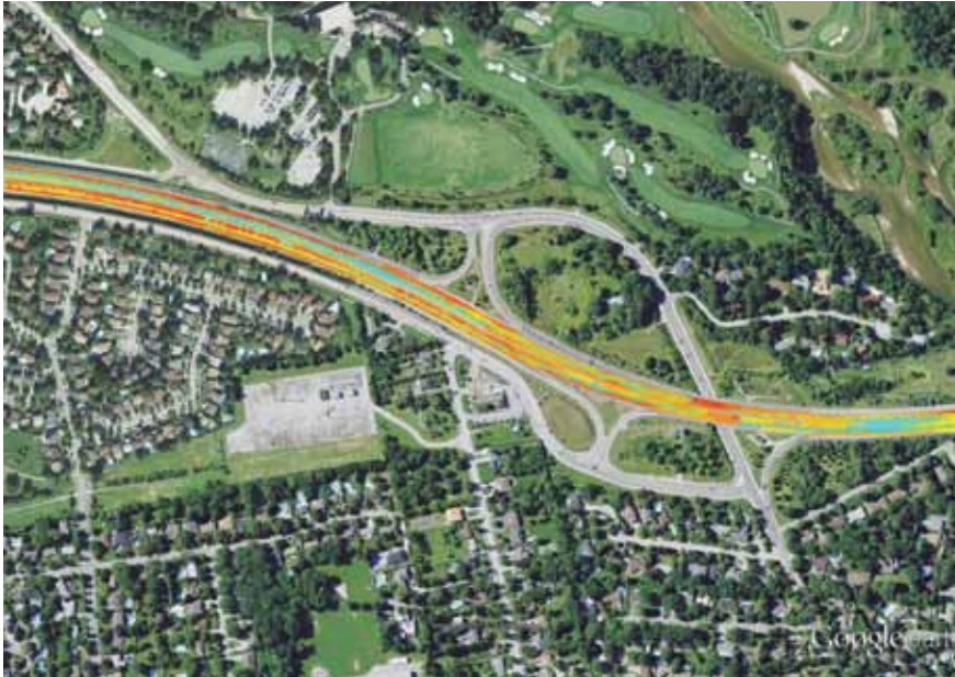
Left: Ground-penetrating radar reveals changes in subsurface properties that allow suspicious areas to be targeted for further evaluation. These areas can then be analyzed and delineated through colour contour maps. Right: Capturing data at posted speeds reduces the impact on traffic flow.
