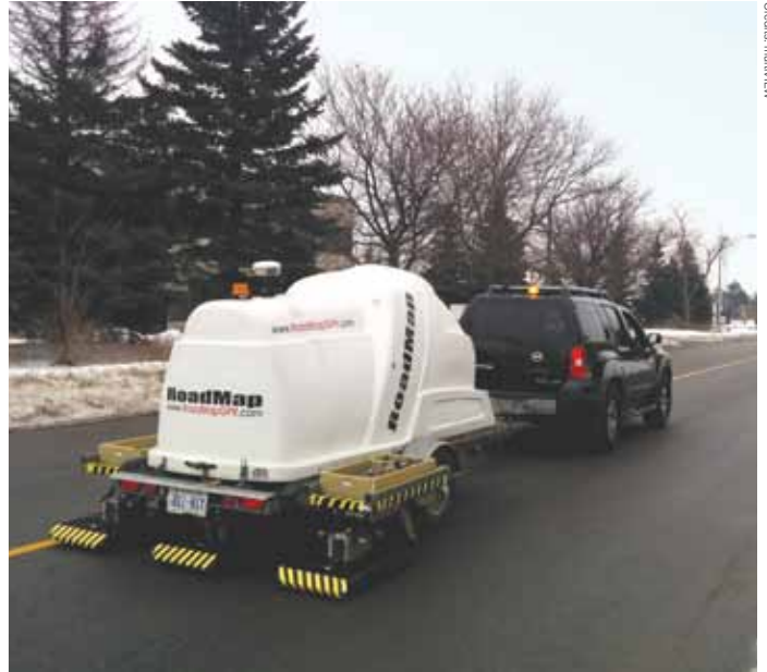
Left: Ground-penetrating radar reveals changes in subsurface properties that allow suspicious areas to be targeted for further evaluation. These areas can then be analyzed and delineated through colour contour maps. Right: Capturing data at posted speeds reduces the impact on traffic flow.
